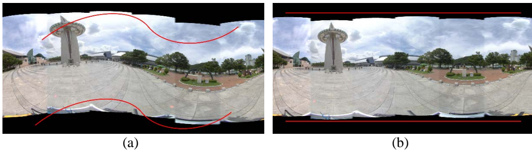
Fig. 4. Contents stitched with VR framework using: (a) scale-invariant features only (without line features); (b) line and scale invariant features. Notice the wavy effect (shown with red wavy lines in (a)) is removed in (b) with the use of line and scale-invariant features.
