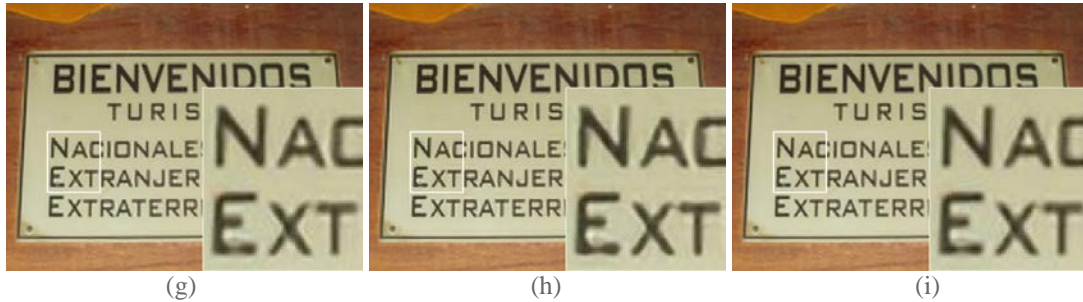
Fig. 6. Visual comparisons with different SR results on indicator by using different methods (magnification factor s = 3 ) (zoom in for better view). (a) Original/PSNR. (b) Bicubic/29.2828. (c) NE + LLE/31.5650. (d) SCSR/30.6459. (e) Zeyde/32.0194. (f) ANR/31.5942. (g) A+/33.2880. (h) SRCNN/33.5718. (i) Proposed/33.6316.
