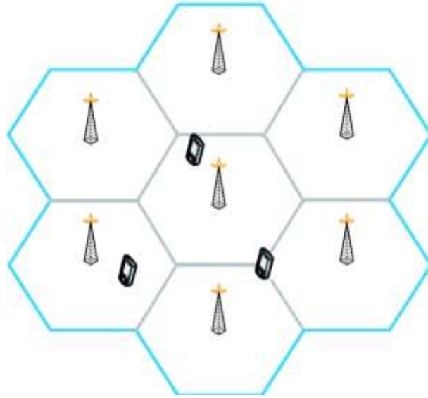
Fig. 1. A predetermined static clustering in multi-cell scenarios
