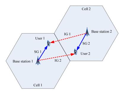
Fig. 2. Two-cell cellular network system model
