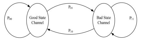
Fig. 5. State transition diagram of two-state Markovian wireless channel
