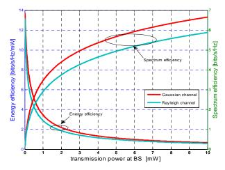
Fig. 1. Relationship between the energy efficiency and spectrum efficiency
