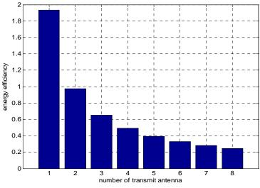
Fig. 6. Impact of number of antennas on energy efficiency
