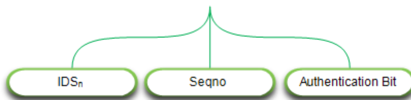
Fig. 4. Cluster Head sends Authentication Packet to CM_s
