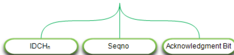
Fig. 3. Cluster Head's sends Acknowledgment Packet to BS
