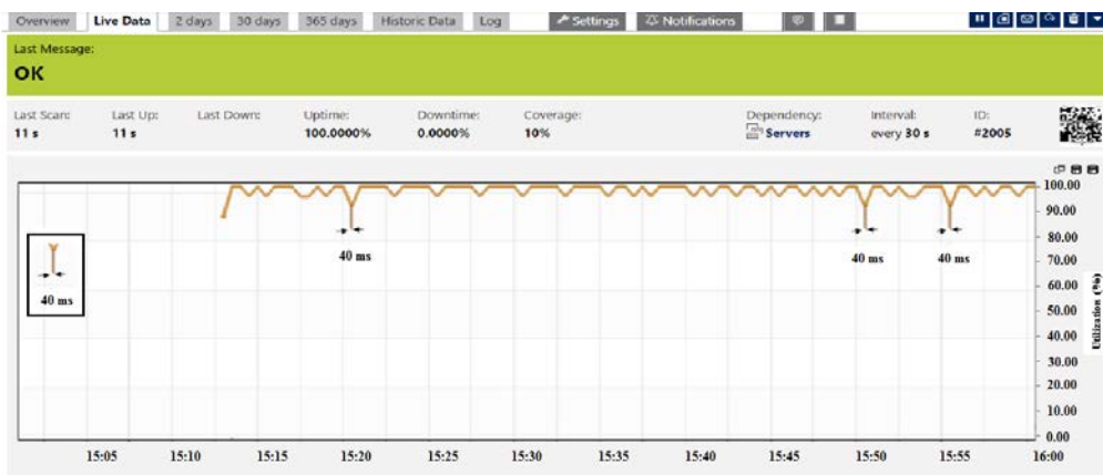
Fig. 16. Transient response (time trace) of the feedback controller in QUEST scheduler
