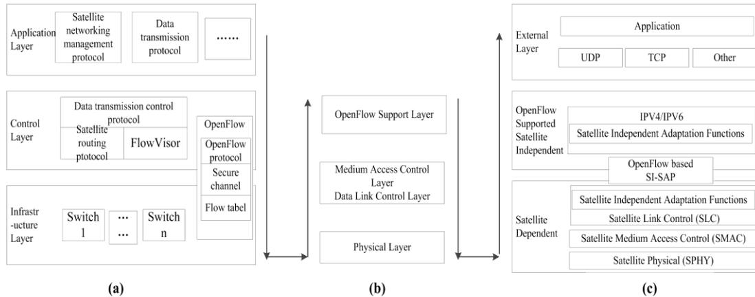
**Fig. 2.** Reference Model of SDOS
