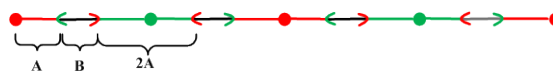
Fig. 7(b). When sensing radius is between L/2 and L , only adjacent sensors' sensing regions will intersect with each other.
