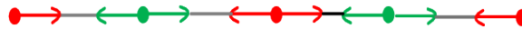
Fig. 7(a). When sensing radius is less than L/2 , sensing regions of all the sensors will not intersect with each other.
