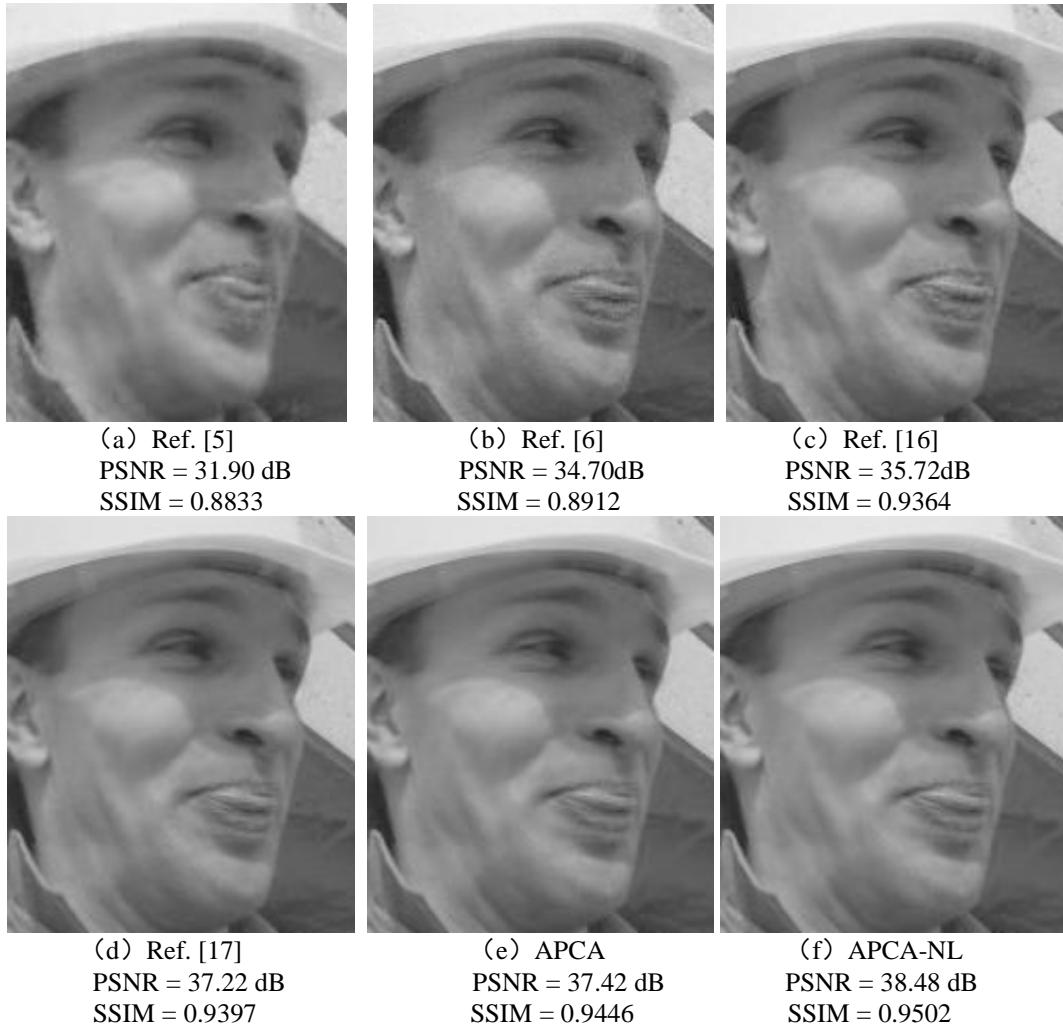
Fig. 5. When S_{NK} is 0.3, the comparison of subjective visual quality on Foreman 8-th frame for various algorithms under I-P-I model.
